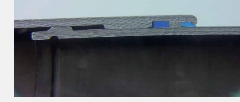
TENIFER® is a salt bath nitriding which produces a thick and homogeneous compounds layer whose structure consists of chemical compounds which are created by a reaction among iron, nitrogen and carbon.
